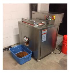
New commercial food dehydrators at the James A. Karnes Corrections Center were installed. As deputies pondered the most earth friendly way to deal with food waste, they settled on this equipment which can reduce food weight and volume by as much as 90-percent. The end product can be used as a soil amendment suitable for use in landscaping
