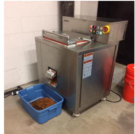
New commercial food dehydrators at the James A. Karnes Corrections Center were installed. As deputies pondered the most earth friendly way to deal with food waste, they settled on this equipment which can reduce food weight and volume by as much as 90-percent. The end product can be used as a soil amendment suitable for use in landscaping
